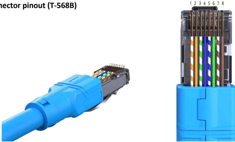
Figure 9 - RJ45 connector pinout
