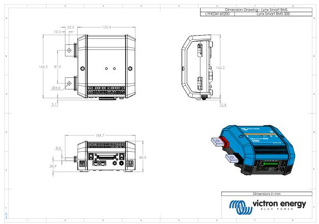
Lynx Smart BMS 500 M8 model enclosure dimensions
