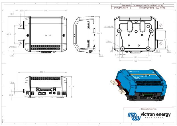
Lynx Smart BMS 1000 M10 model enclosure dimensions
