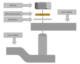
Connection sequence when connecting two Lynx modules
