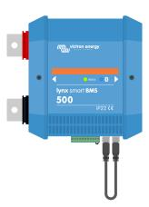
Testing a Lynx Smart BMS by connecting a single BMS extension cable to both BMS cable connections
