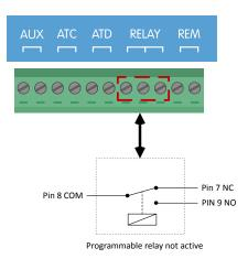
Pinout for the programmable relay
